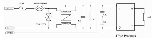
Fuse: recommended parameters: 5A to 10A/250Vac, Time-lag type.
