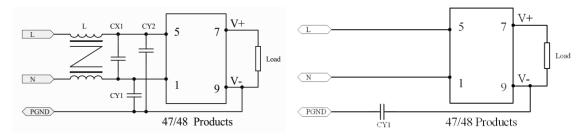
L is a common mode inductor, recommended parameters: 10mH to 30mH CX1 is a X2 capacitor, recommended parameters: 0.1uF to 0.22uF/275Vac CY1 and CY2 are Y capacitors, recommended parameters: 1000pF to 2200pF/400V
